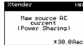
**i** In case of using the Xtender on a public grid, it is actually the value of the circuit breaker on the source side (fuse or breaker).
