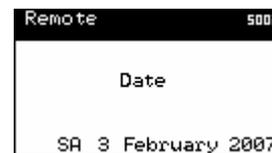
Set the correct date using the keys UP and DOWN
